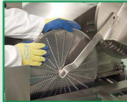
Quick and easy shred disc changeover
