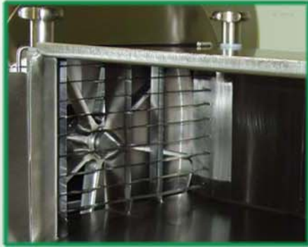
Removable precut blades to adjust length
