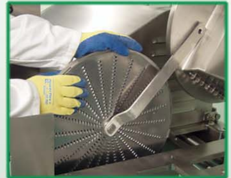
Quick and easy shred disc changeover
