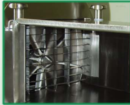
Removable precut blades to adjust length
